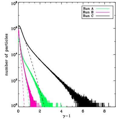
Fig. 3. Energy spectra of the electron in the downstream region. The results are compared for (a) Run A (green), Run B (magenta), and Run C (black). Dashed lines are fitted Maxwell distributions.
