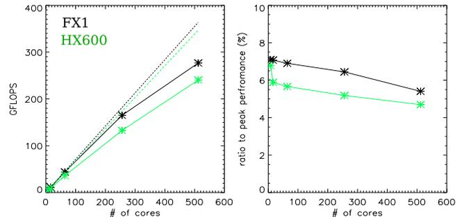
Fig. 1. (Left) Performance of the PIC code in GFLOPS vs. number of processor cores. Solid and dashed lines with symbols are the obtained results for Fujitsu FX1 and Fujitsu HX600, respectively. The straight lines indicate 100% efficiency of the parallelization. (Right) Efficiency of the performance vs. number of processor cores.
