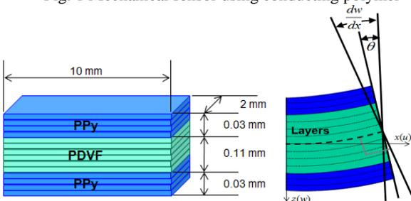
Fig. 2 Layered Timoshenko beam model
