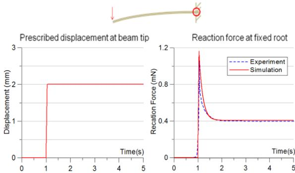
Fig. 3 Time history of tip displacement and reaction force
