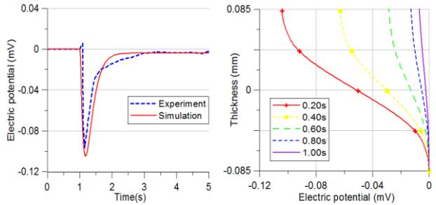
Fig. 6 Electric potential output with respect to time(left) and electric potential over thickness at root(right)
