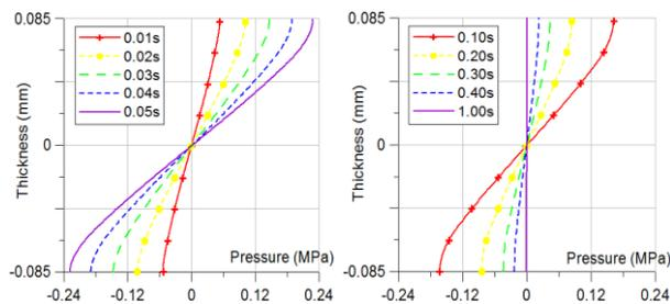
Fig. 4 Pressure distribution over thickness at beam tip during loading(left) and relaxation(right)
