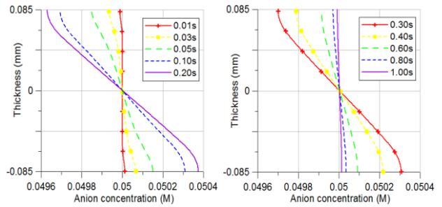
Fig. 5 Mobile ion concentration over thickness at beam root during loading(left) and relaxation(right)
