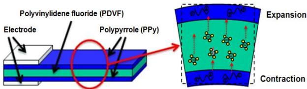
Fig. 1 Mechanical sensor using conducting polymer
