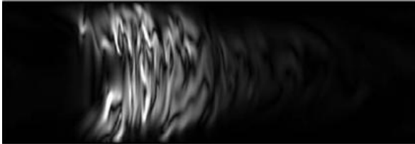
(a) The turbulent puff structure in a pipe flow.
