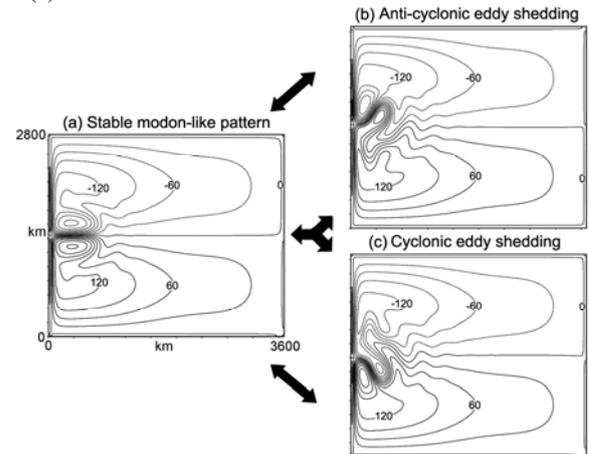
**Figure 5** Three typical flow patterns (monthly averaged 1st layer thickness,  $CI=30m$ ) of double gyres in Q-G model for  $\alpha = 0.7$ . (a) Stable modon-like pattern, (b) anti-cyclonic eddy shedding, and (c) cyclonic eddy shedding.
