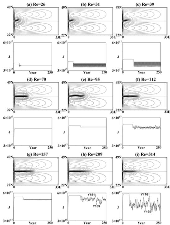
**Figure 1** Average flow patterns (1st layer thickness, upper panels) and time series of total energy (lower panels) for (a)  $Re = 26$ , (b)  $Re = 31$ , (c)  $Re = 39$ , (d)  $Re = 70$ , (e)  $Re = 95$ , (f)  $Re = 112$ , (g)  $Re = 157$ , (h)  $Re = 209$  and (i)  $Re = 314$ . The periods indicated by arrows in (h) and (i) are included in those of Fig. 2.
