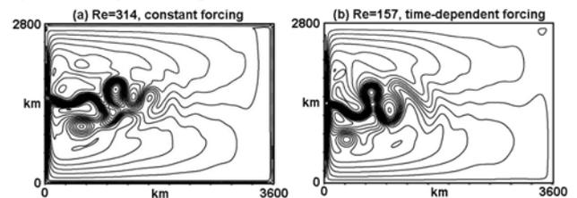
**Figure 6** Flow patterns (monthly averaged 1st layer thickness,  $CI=20m$ ) for (a)  $Re=314$ , constant forcing at 86 years, 11 months and (b)  $Re=157$ , time-dependent forcing at 184 years, 3 months.
