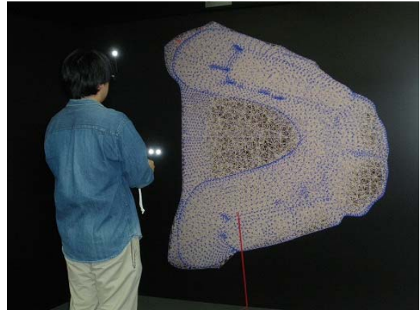
Fig. 5 Mesh modification using controller in VR space
