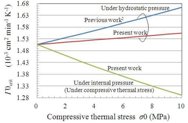
Fig. 3 Variations in critical  $v/G$  ( $v$ : pulling speed,  $G$ : temperature gradient) ratio  $\Gamma_{crit}$  with thermal stress  $\sigma_0 = P_{in}$ . Results obtained by using values for  $H_f$  and  $H_m$  under hydrostatic pressure  $P_h$  are also given.
