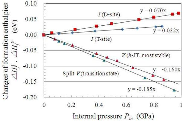
Fig. 2 Changes in formation enthalpies  $\Delta H_f^I$  for D-site (most stable) and T-site (transition state),  $\Delta H_f^V$  for Jahn-Teller distortion ( $h$ -JT, most stable) and split- $V$  (transition state) due to internal pressure  $P_{in}$ .
