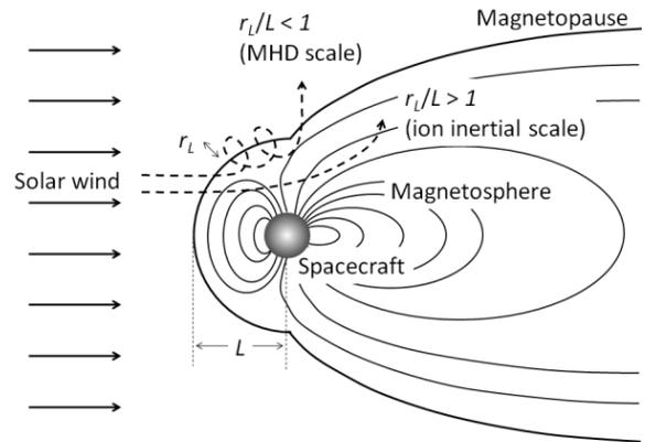
Fig. 1. Ion particle motion due to the difference on  $r_L/L$ .
