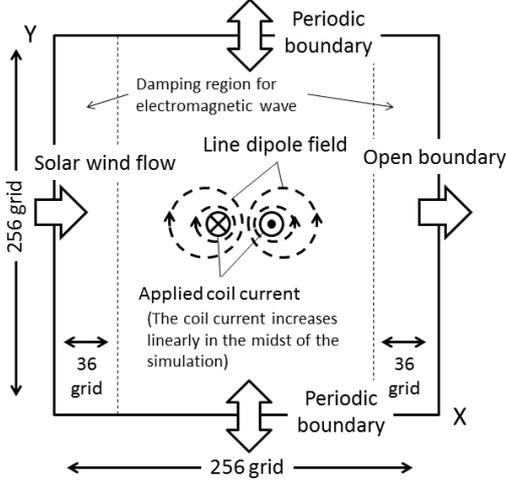
Fig. 3. Computational domain used in the two-dimensional AMR-PIC simulation.
