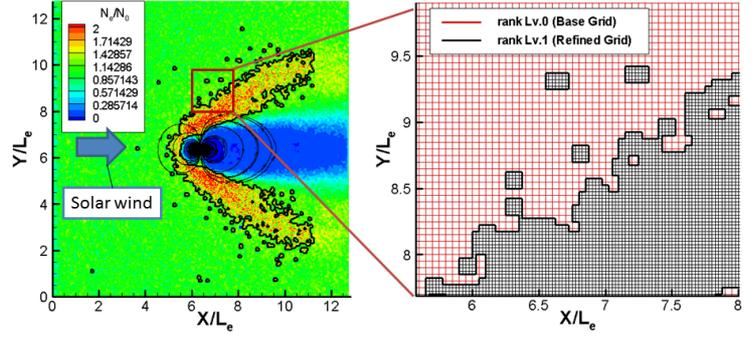
Fig. 4. Distribution of the electron number density, magnetic field lines and refinement grid at  $t = 10 [1/\omega_{pe}]$
