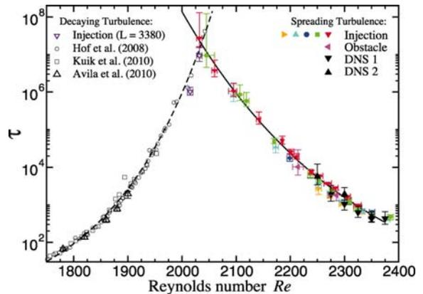
Fig. 2: Mean lifetime of a puff.<sup>[2]</sup> Dashed and solid curves represent decaying and splitting time respectively.
