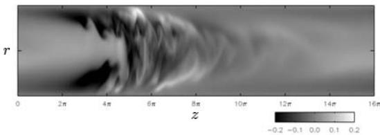
Fig. 1: Turbulent puff in pipe flow.<sup>[1]</sup> Gray scale represents perturbation velocity,  $u_z - \langle u_z \rangle_{\theta z}$ , in a plane through the pipe's centerline.
