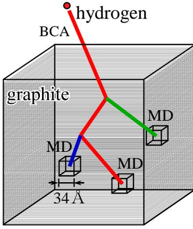
Fig. 1. Schematic diagram of the BCA-MD hybrid simulation of hydrogen injection into a graphite.[3]
