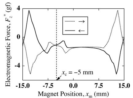
Fig. 4. Spatial distribution of the electromagnetic force  $F_z^*$  for  $L_c = 0.83$  mm and  $x_c = -5$  mm. Here, two types of arrows indicate the scanning direction of the magnet.
