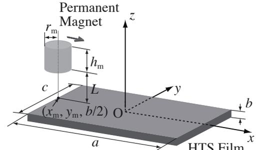
Fig. 1. A schematic view of a scanning method.
