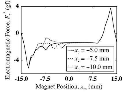
Fig. 3. Spatial distribution of the electromagnetic force  $F_z^*$  for  $L_c = 0.83$  mm.
