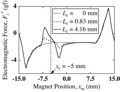
Fig. 2. Spatial distribution of the electromagnetic force  $F_z^*$  for  $x_c = -5$  mm.
